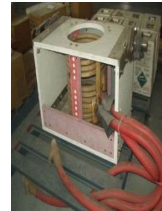
RS-100 is used as a structural component in the construction of induction melters.
