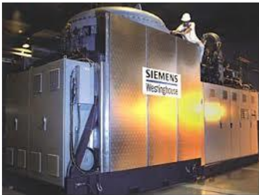
Siemens Solid Oxide Fuel Cell.
