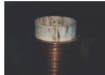
RS-101 is used as a coil liner for coreless induction melters.
