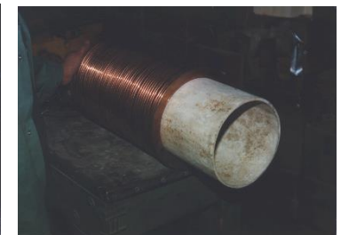
RS-101 is used as a coil liner for coreless induction melters.
